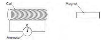
The ammeter has a centre zero scale, so that values of current going in either direction through the coil can be measured.
